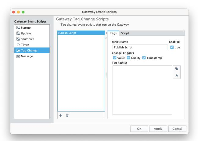
After setting the name of the script and then select a tag path. In this case we're using a tag in the default tag provider called 'MyTriggerTag' as shown below.
