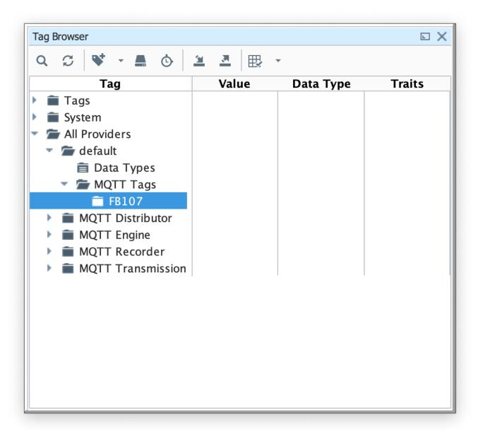
Note this structure is based on usage of the 'Example Transmitter' in MQTT Transmission in Ignition8. So, the directory structure is very important. Note the structure
