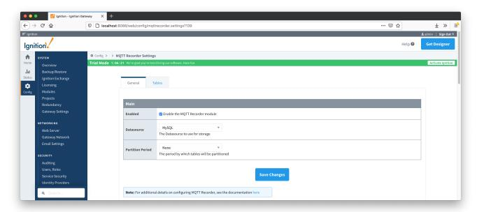
At this point, the Central Ignition Gateway with MQTT Distributor, MQTT Engine, and MQTT Recorder is fully configured and ready to receive MQTT Sparkplug messages from the Remote/Edge Ignition Gateway. MQTT Distributor listens on TCP port 1883 by default for inbound MQTT connections. Make sure the Operating System's Firewall, Antivirus, and Malware protection services allow inbound connections on port 1883/TCP before proceeding.
