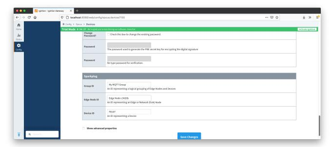
Next the MQTT Transmission server configuration must be modified to point to the Central Ignition Gateway we set up earlier. To do so, in the Ignition Gateway Web UI browse to the Configure tab on the top and then to MQTT Transmission Settings in the lower left as shown below.
