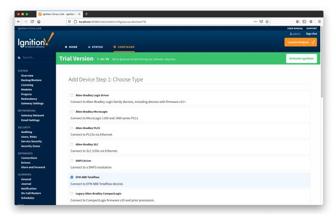
This opens the 'New Device' configuration mage for ABB Totalflow Device:
