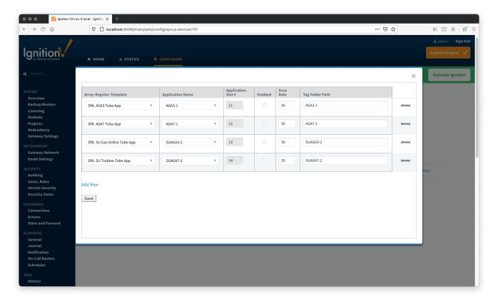
When this is done, the 'Devices' configuration page will show the 'Status' for each device changed from 'Connected' to the 'Polling' state.
