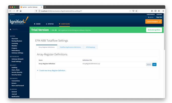
New Array-Register Definitions can be created by following the 'Create new Array-Register Definition' link as shown below:
