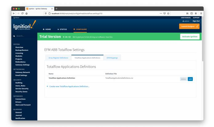
A new Totalflow Applications Definition can be added by clicking on the "Create new Totalflow Applications Definition..." link.
