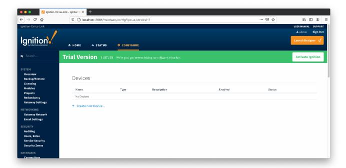
New ABB Totalflow device can be created by following the 'Create new Device...' link and choosing 'EFM ABB Totalflow' device as shown below:
