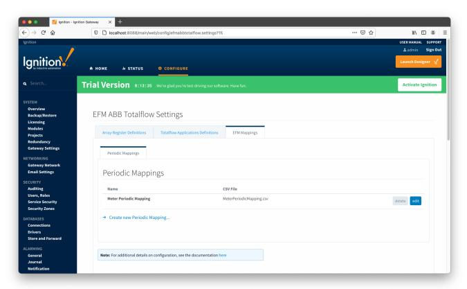
A new Periodic Mapping can be added by clicking on the "Create new Periodic Mapping..." link.
