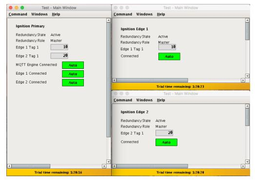
At this point we can begin failing Ignition instances. From the Status Redundancy page we can use the 'Force Failover' button as shown below. Of course stopping the actual Ignition instance is another option.
