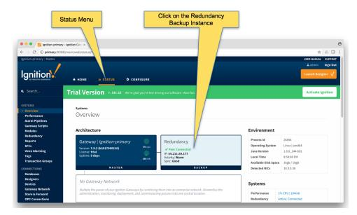
Force the Re-sync via the button below. This will duplicate the master configuration to the backup Ignition instance it is connected to.
