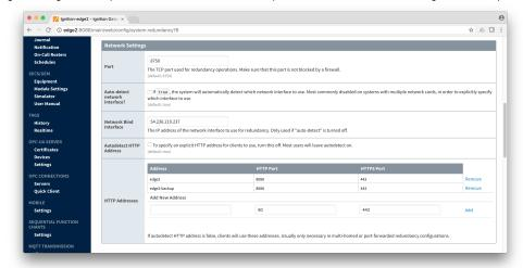
Set the Master Node Address. Note in the configuration below a hostname is being used. This should be the primary network interface address of the Ignition Edge 2 Gateway.
