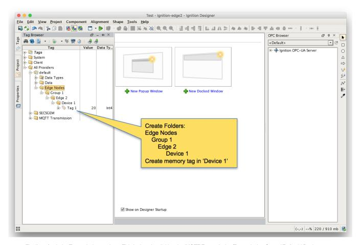
• Finally, refresh the Transmission runtime. This is done by clicking the 'MQTT Transmission/Transmission Control/Refresh' Boolean tag.
