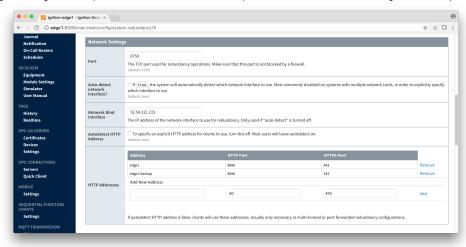
Set the Master Node Address. Note in the configuration below a hostname is being used. This should be the primary network interface address of the Ignition Edge 1 Gateway.
