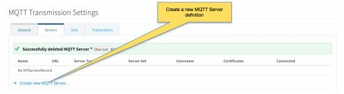
Configure MQTT Transmission to point to the Primary Ignition. Configure as shown below making sure to change the URL to reflect your network settings. For example, if you Ignition Primary is at 192.168.1.100 the MQTT Server URL would be: tcp://192.168.1.100:1883. Af ter setting the parameters as shown below. Click the 'Save Changes' button at the bottom.
