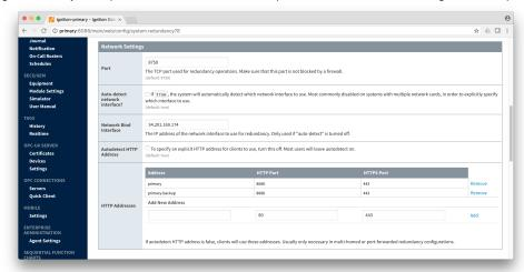
Set the Master Node Address. Note in the configuration below a hostname is being used. This should be the primary network interface address of the Ignition Primary Gateway.
