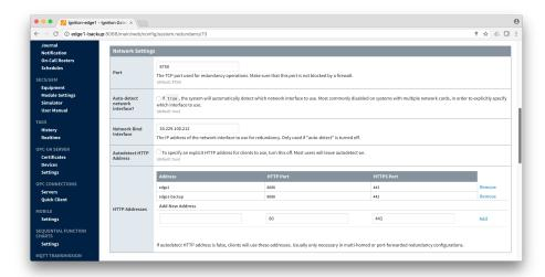
Set the Master Node Address. Note in the configuration below a hostname is being used. This should be the primary network interface address of the Ignition Edge 1 Gateway.
