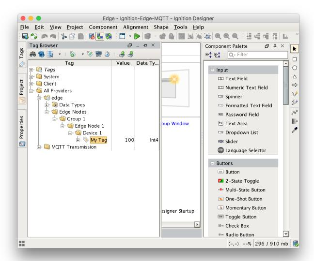
Note additional tags could be added to the 'Device 1' folder as well. These could be OPC tags, UDTs, or other types of tags. Also, additional folders could be added below this level as well. The structure of the 'default transmitter' requires that the first three folder levels represent the Sparkplug Group ID, Edge Node ID, and Device ID respectively.
