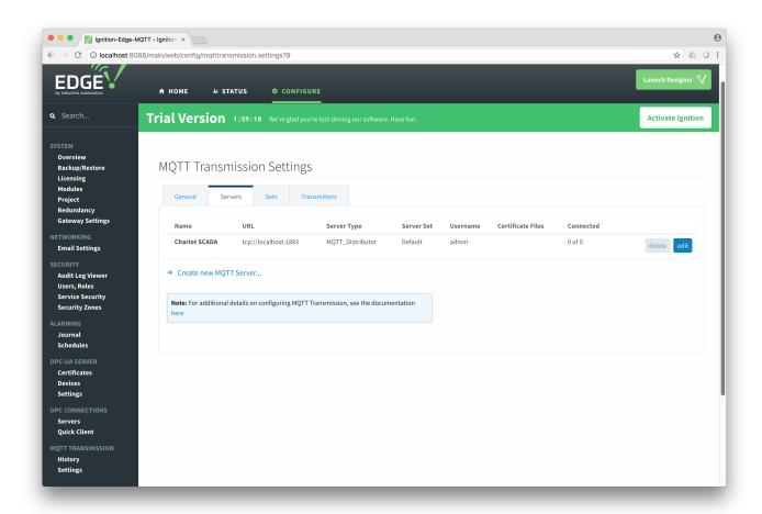
At this point, modify the URL to point to the Central Ignition Gateway's IP address. For example, if you central Ignition gateway is at 10.10.10.123, set the URL to tcp://10.10.10.123:1883. Then save your settings.
