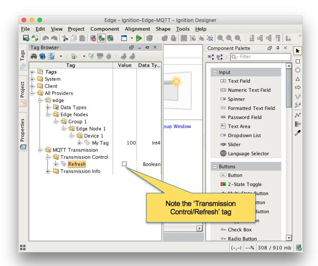
Step 6: Verify MQTT Transmission is Connected
