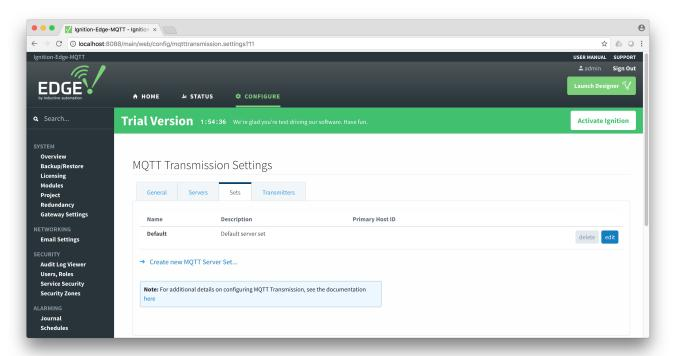
Now set the 'Primary Host ID' to the same ASCII string that was set in MQTT Engine previously as shown below and save the changes.
