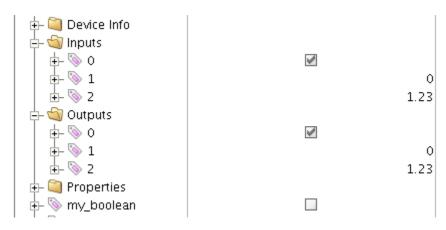
You should see the Tag value change as well as the value of the corresponding Tag in the Inputs folder. In the Sparkplug example code the outputs are virtually tied to the inputs. So, when modifying an output value, this causes an MQTT message to be sent from MQTT Engine, to the virtual device, which receives the message, modifies the values, and then publishes a MQTT message back to MQTT Engine where the two values are updated.
