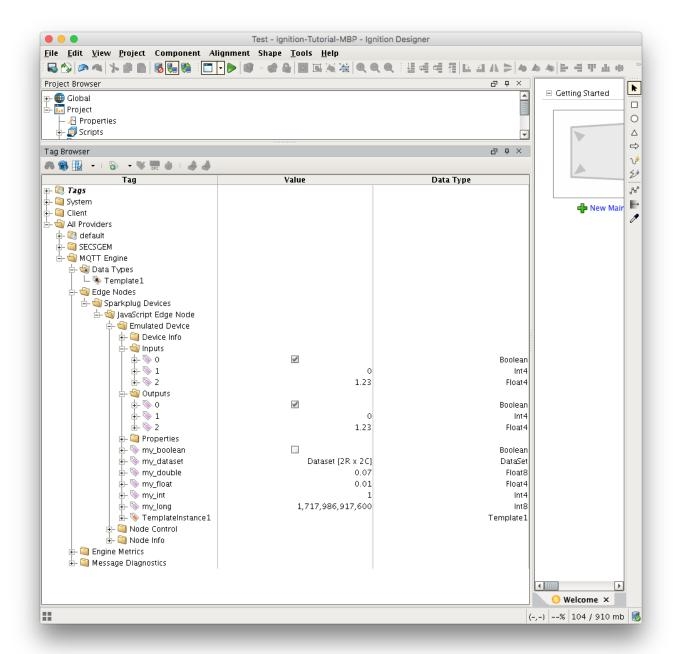
You will see that MQTT Engine saw a new device attach to the MQTT Server and publish a Birth Certificate. As a result, MQTT Engine created the Ignition Tags shown above. These are also dynamically updated as the values change. You can also write to the outputs after you Enable Device Writes from Ignition. This can be done by putting designer into read/write mode.
