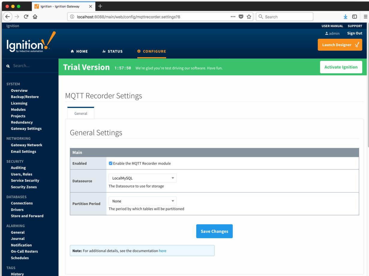
At this point, the Central Ignition Gateway with MQTT Distributor, MQTT Engine, and MQTT Recorder is fully configured and ready to receive MQTT Sparkplug messages from the Remote/Edge Ignition Gateway. MQTT Distributor listens on TCP port 1883 by default for inbound MQTT connections. Make sure the Operating System's Firewall, Antivirus, and Malware protection services allow inbound connections on port 1883/TCP before proceeding.
