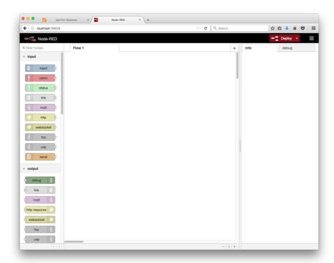
We need to install the node-red-contrib-sparkplug library module into Node-RED. We can do this using the "Manage palette" option in the upper right dropdown menu.
