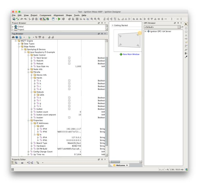
You will see that MQTT Engine saw a new device attach to the MQTT Server and publish a Birth Certificate. As a result, MQTT Engine created the Ignition Tags shown above. These are also dynamically updated as the values change. You can also write to the outputs after you Enable Device Writes from Ignition. This can be done by putting designer into read/write mode. Do so by clicking this button in the menu to enable read/write mode:
