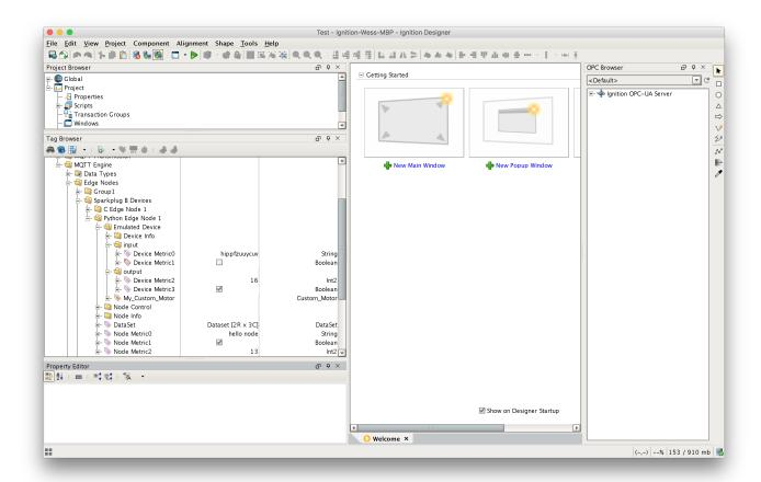
You will see the result of MQTT Engine seeing a new edge node and device connect to the MQTT Server and publish an NBIRTH and DBIRTH message. As a result, MQTT Engine created the Ignition Tags shown above. These are also dynamically updated as the values change. You can also write to the outputs after you Enable Device Writes from Ignition. This can be done by putting designer into read/write mode. Do so by clicking this button in the menu to enable read/write mode:
