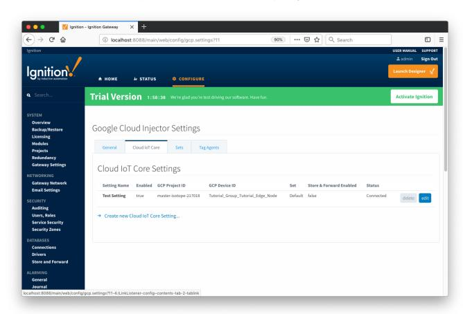
One or more Cloud IoT Core endpoints can be configured on this tab. The configuration options for a Cloud IoT Core connection are listed below.
