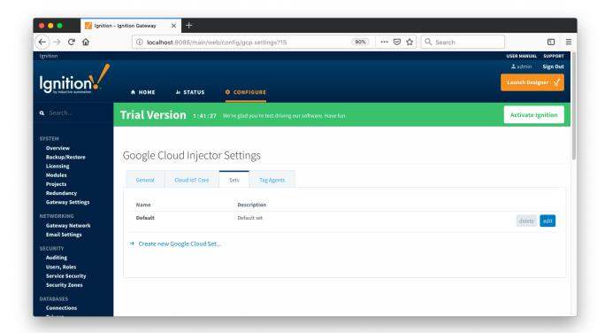
Additional Sets can be configured for situations where multiple Tag Agents will need to push to different Cloud IoT Core endpoints. The configuration options for Sets are listed below.
