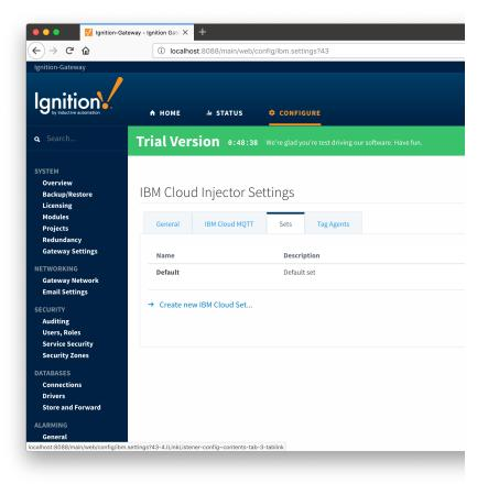
Additional Sets can be configured for situations where multiple Tag Agents will need to push to different IBM Cloud MQTT endpoints. The configuration options for Sets are listed below.
