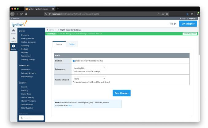
At this point, the Central Ignition Gateway with MQTT Distributor, MQTT Engine, and MQTT Recorder is fully configured and ready to receive MQTT Sparkplug messages from the Remote/Edge Ignition Gateway. MQTT Distributor listens on TCP port 1883 by default for inbound MQTT connections. Make sure the Operating System's Firewall, Antivirus, and Malware protection services allow inbound connections on port 1883/TCP before proceeding.
