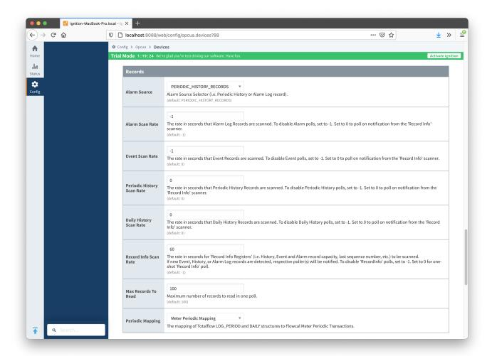
At this point the EFM ABB Totalflow driver is configured and is polling for history data at the rate specified in the EFM ABB Totalflow device configuration.
