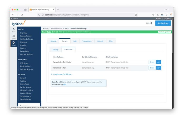
Update the MQTT Transmission > Servers > Settings configuration to use the certificates as shown below. Click the Save Changes button to save the configuration. Note the URL must use SSL. If a non-secure connection is specified here, the connection will not succeed.
