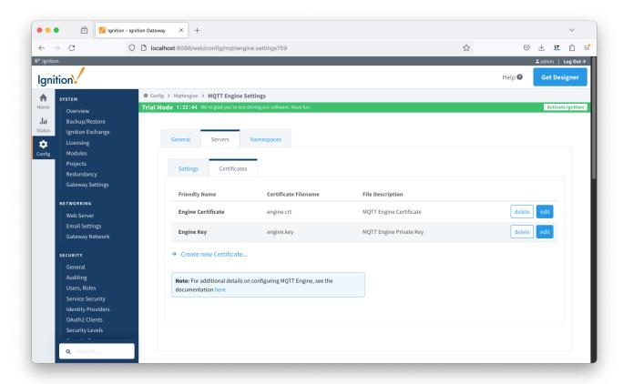
Update the MQTT Engine > Servers > Settings configuration to use the certificates as shown below and setting the URL to be ssl://FQDN:8883 with the FQDN of the Chariot Server. Click the Save Changes button to save the configuration. Note the URL must use SSL. If a non-secure connection is specified here, the connection will not succeed.
