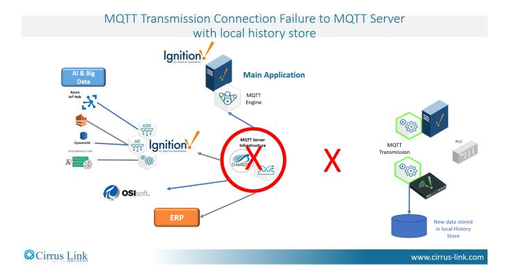
When used in connection with a **Primary Host ID** we can also ensure data is also buffered locally in the event the main application is offline. The primary host ID identifies the main application that is receiving the MQTT data from the MQTT Server and is used by the edge node to subscribe to state notifications for that application.
