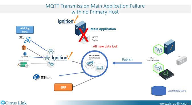
If the primary host ID is configured and there is a change to the connection status with the main application, the MQTT Server will publish a state message to clients which have subscribed to this state message. When connected the status will be ONLINE and when disconnected the status will be OFFLINE.
