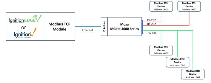
The gateway uses male DB9 serial ports to connect to the Modbus RTU or ASCII devices.
