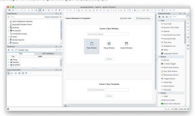
Deselect Sample\_Tags and select MQTT Engine under the Tag Browser window. Expand the Edge Nodes folder tree until you have exposed the PLC 1 folder with the Example Tag.
