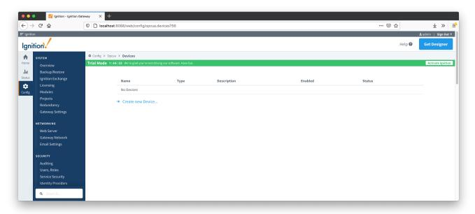
A new Opto 22 groov EPIc and SNAP PAX device can be created by following the 'Create new Device...' link and choosing 'Opto 22 groov EPIC and SNAP PAC' device as shown below:
