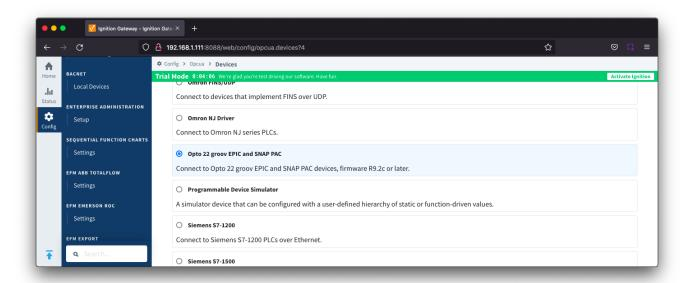
This opens the 'New Device' configuration page for Opto 22 groov EPIC and SNAP PAC Device. The configuration sections available are General and Opto 22 groov EPIC and SNAP PAC Settings.
