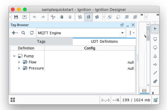
From the Designer connected to the Edge1 instance, make changes to the Stream1 tag Flow and Pressure member tags and see the data published and displayed on the MQTT engine instance of Designer.
