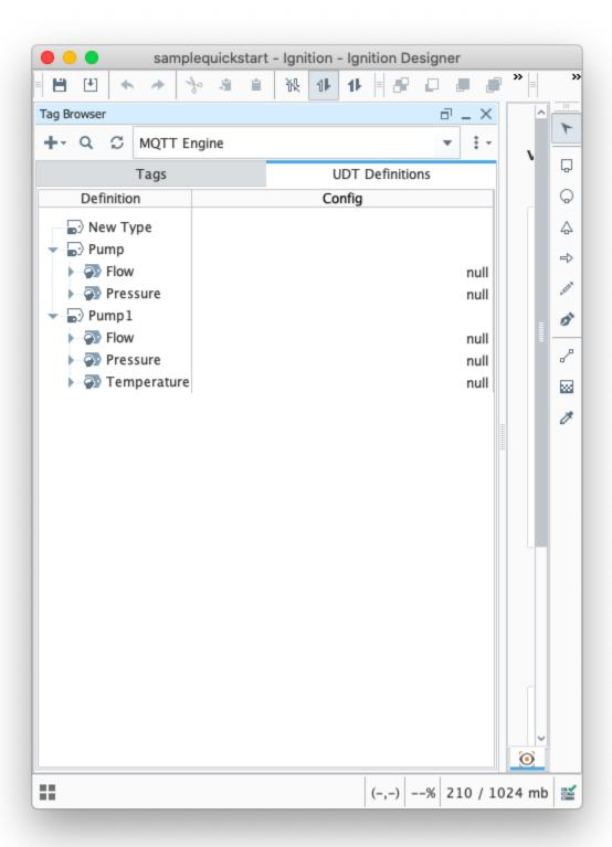
Once the new definition is created, you can create an instance on the edge device and force the refresh. The new UDT definition will be recorded by MQTT engine and the data processed correctly without impacting the data published from other edge devices. The system can run like this indefinitely with the updated definition imported into any other locations that need to use that new definition.
