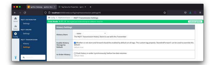
Note: Store and Forward does not guarantee all data is stored and forwarded. There are some edge cases that are not currently handled with regard to data loss in the event of connection failures related to MQTT keep alive timeouts. This window of potential missed data can be reduced by decreasing MQTT Transmission and MQTT Engine configurable keep alive timeouts.
